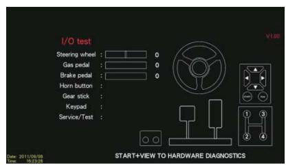
2 Enter the page of [I/O test], you can run testing for a specific application as explained in the chart below:
