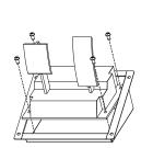
Then loosen the four M8 cruciform screws, and replace the whole set. When completed, resemble according to the reversed assembly sequence.
