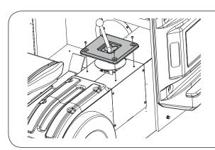
Loosen the four M5 inner hex screws to unload the cap.
