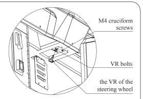
Then loosen the M4 cruciform screws and VR bolts. After the VR of the steering wheel is replaced, resemble according to the reversed assembly sequence.
