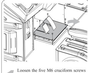
Loosen the five M6 cruciform screws to unload the cap, holder, and the connector.
