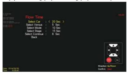
② After the settings is completed, move the cursor to [Back] and press the [START] button to leave this page.
