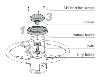
Loosen the three M4 inner hex screws to unload the holder.
