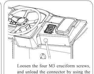
control pad. When completed, resemble according to the reversed assembly sequence.
