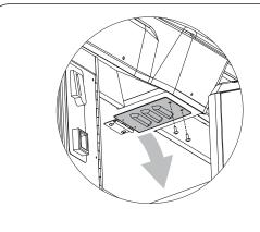
Loosen the two cruciform screws to open the maintenance door.
