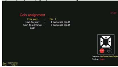
3 When the setting is completed, move the cursor to [Back], and press the [Start] button to leave this page.
