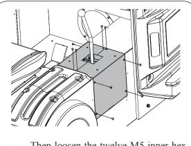
Then loosen the twelve M5 inner hex screws to open the maintenance door on both sides.
