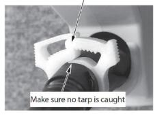
Move the clamp from step 14 down along the tarp to about 1 to 1.5 cm from the hole. Checking that none of the tarp is caught in the clamp, and that the interlocking portion of the clamp is still facing the handle of the controller, tighten the clamp as far as it will go, using pliers or a similar tool.
