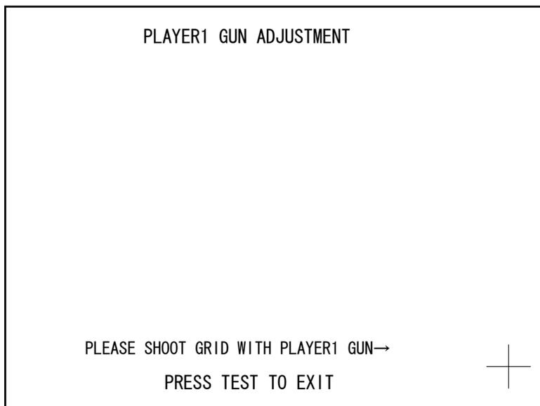
Aim and fire at the mark to the lower right. The mark to the lower right will disappear, and the same mark will be displayed in the center.
